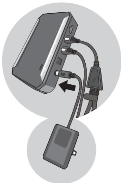
**1** Insert the cord extending from the module into the port marked "MFP" on the control box.
