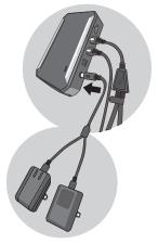
Unplug any modules already installed in the port marked "MFP"
