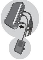
Insert the cord extending from the module into the port marked "MFP" on the control box.
